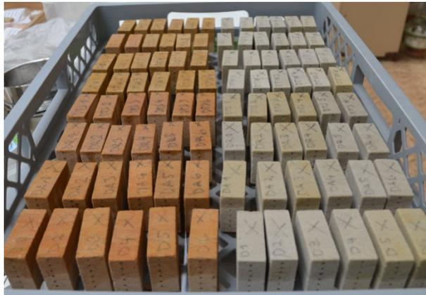
Fig. 41. Treated samples' storage in natural climatic conditions
