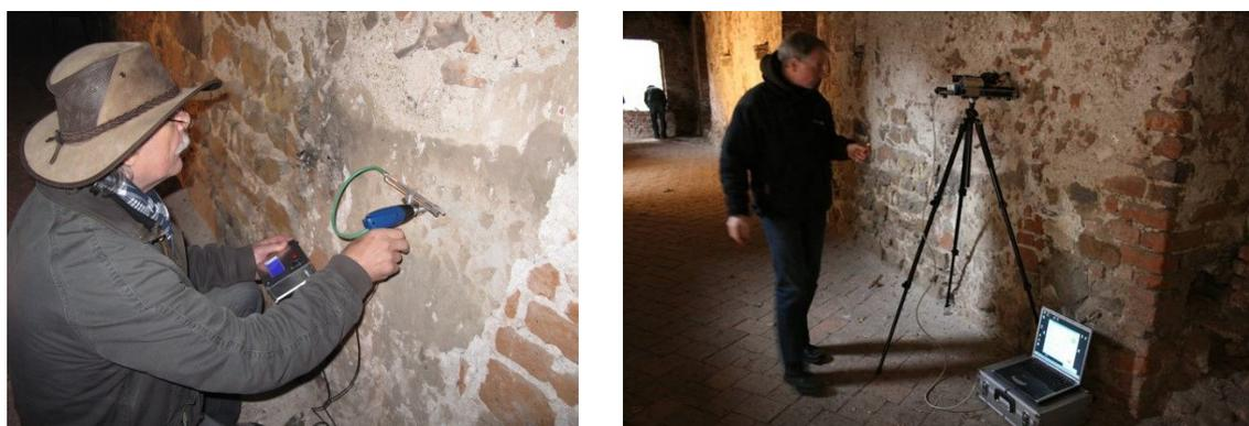
Fig. 6 In situ testing of the plaster parameters: water absorption rate by means of micro-tube (left) and drilling resistance using DRM system (right).
