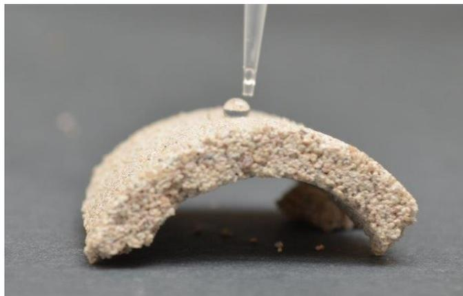
Figure 19 Test of the water drop absorption rate
