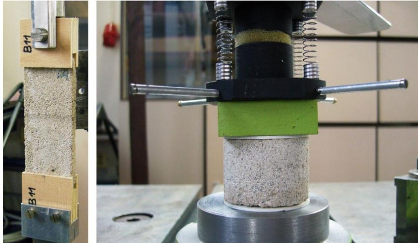
Fig. 7 Testing specimens - thin plates for tensile tests (left) and tubes for compressive test (right)
