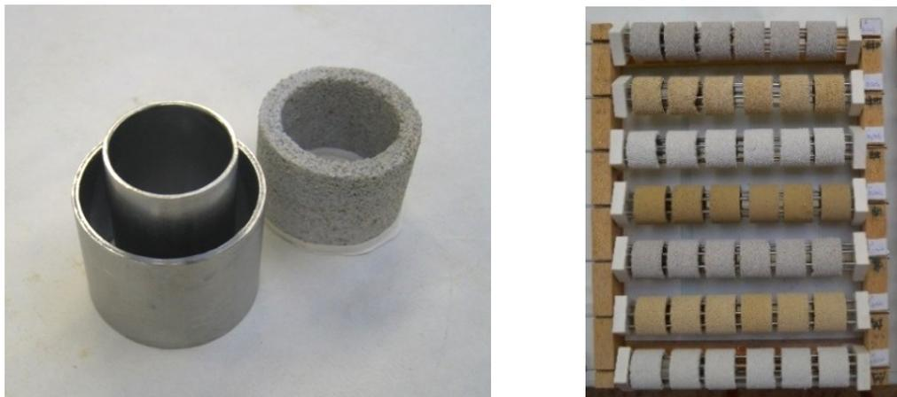
Fig. 21 Mortar tubes: specimen production (left) and arrangement of the consolidation treatment
