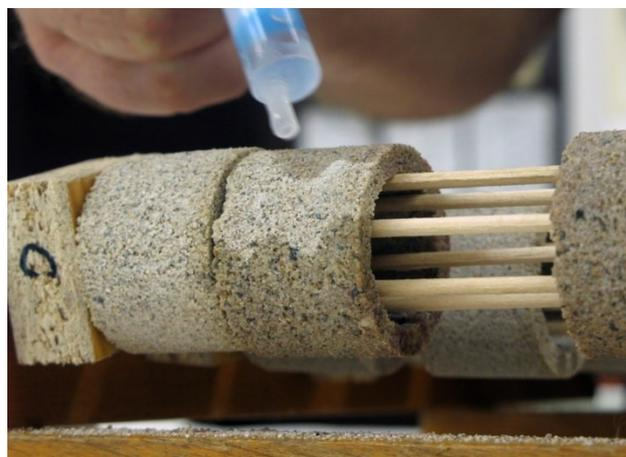
Figure 8. Impregnation of short tubes, using a syringe
