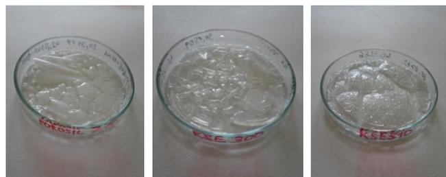
Fig. 50 Structures of gels formed from the consolidants tested after 1 week.
