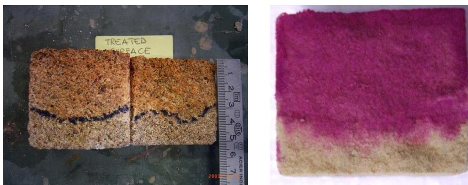
Fig. 4 a,b Use of indicator liquids to assess the presence of a product in a substrate. Left – dithizon, used for ethyl silicate; right – phenolphthalein used for the assessment of the penetration of a nanolime consolidant [Borsoi G. et al. 2015]
