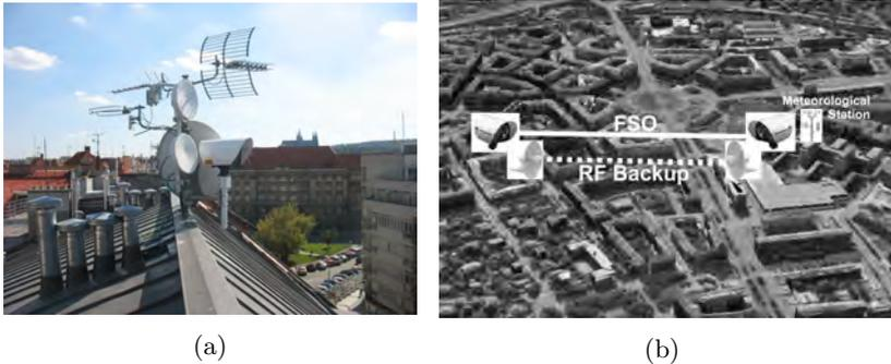
Figure 10: a) FSO/RF transmitting site at the Orlik dormitory; b) experimental campaign arrangement for RF/FSO
