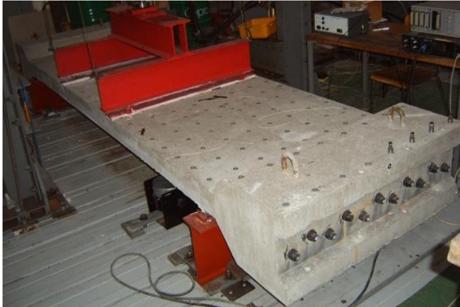
Figure 4: The view on the slabs concreting and the position of the slab in the loading stand.
