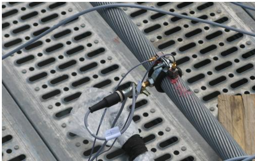
Figure 2: The view on the vibration transducers (accelerometers) installed on the cable.
