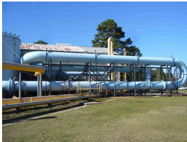
Figure 2 Example of laboratory loops for slurry-flow testing: GIW Industries loops for slurry-pump testing (larger loops, blue), and slurry-pipe testing (smaller loops, yellow)
