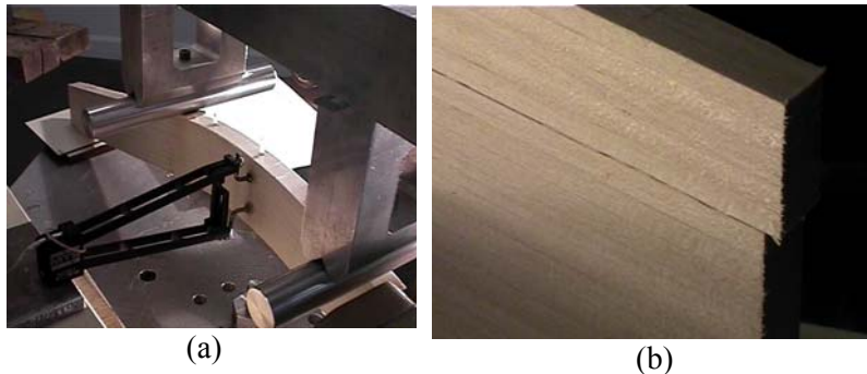
Figure 1. Bending test of curved beam with radial reinforcement [1]. (a) Test setup, and (b) failure of an unreinforced beam due to the radial crack propagation.
