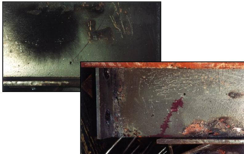
*Fig.11: Fatigue cracks in the steel grid*
