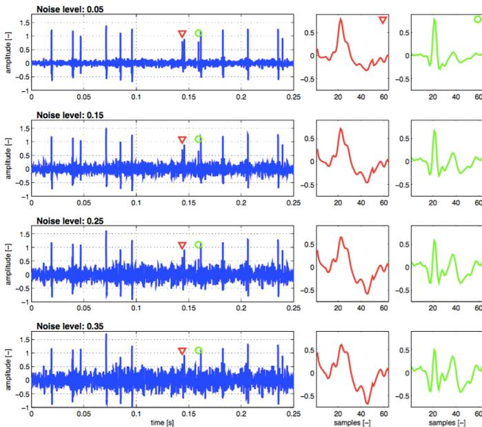
Figure 3: Example of spike detection with different noise levels ranging from 0.05 to 0.35. The spikes marked in the signal by a triangle and a circle each belonged to a different neuron and are shown in greater detail on the right side - in the case of a higher noise level at 0.25 and 0.35, a new noisy spike could be misleadingly detected. [Wild et al., 2012]
