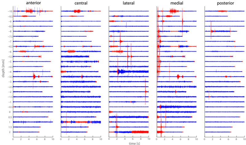
Figure 2: Example of artifact detection on MER recordings with five parallel electrode trajectories. [Bakstein, 2017]
