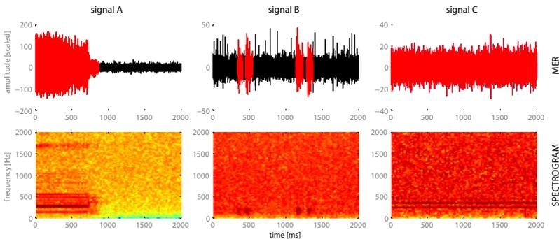
Figure 1: Two second samples of the most commonly inspected artifacts: raw MER signal with artifact regions in red (top row) and corresponding spectrogram (bottom row). Signal A) shows intermittent electromagnetic interference, signal B) mechanical artifact and signal C) uninterrupted electromagnetic interference at 235 and 350 Hz. [Bakstein, 2017]
