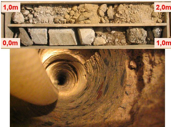
Fig. 10 Core samples extracted from the MPD04A borehole and view to the borehole before deployment of the measuring casing and grouting (grouting tube on the left of the photo).
