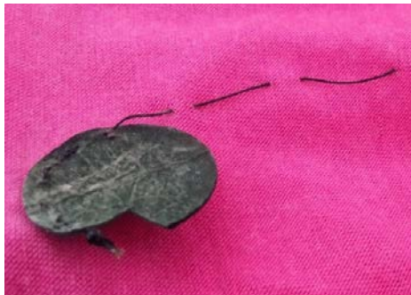
Figure 5: Implemented flat electrode and textile polymer-based conductor on elastic material
