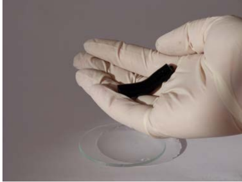
Figure 4: Ready underlying textile material coated with a layer 100 nm layer of electrically conductive polyaniline
