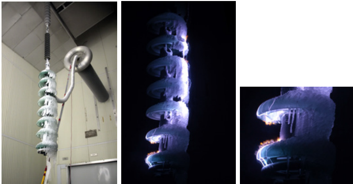
Figure 16: Tested insulator string after the ice accumulation stage (left), the arc trajectory (middle) and the detail of the arc trajectory for two bottom insulators (right)
