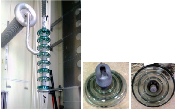
Figure 13: Test circuit for insulator in climatic chamber
