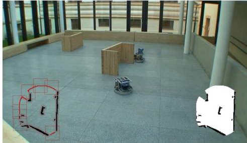
Figure 2: Two robots in an experimental evaluation of the multi-robot exploration. The small superimposed map on left is visualization of the current frontiers while on right is shown the the current grid map of the explored part of the environment.
