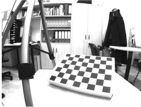
Fig. 2.7: Radial distortion of the image.
