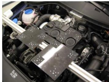
*Fig. 4.3: Multi-camera measuring system for dynamic capture of engine movements or movements of any fixed bodies (left). Mounting frame for car reference points on engine block and vehicle (right) [1].*
