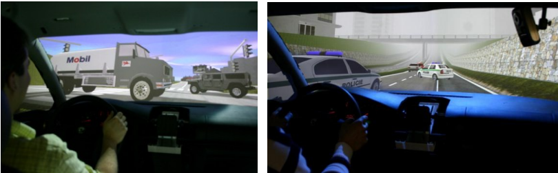
Fig. 19: The shadow cast by the truck moving around the simulated car (left) and dynamic scattered blue light is emitted by police car beacons (right)
