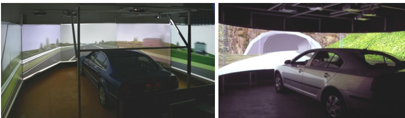
Fig. 25: Superb simulator upgraded with 5 projectors surrounding projection screens (2006) – left and driving simulator Octavia II (2008) - right
