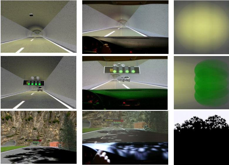
Fig. 20: Examples of the objects, their projection on the real cockpit and their casting maps (from the top to the bottom: Tunnel driving, Traffic lights in the dark environment, Open scenery with trees)
