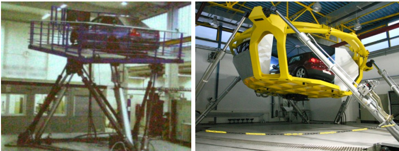
Fig. 7: Full car simulator situated on robust hexapod platform in BMW – left and one of the European latest simulators by Simtec and DLR – right
