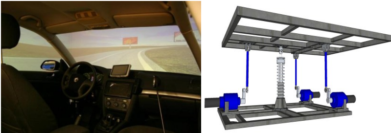
Fig. 26: Cockpit of the light simulator Octavia II 3D (2010) (left) and 3DOF moving platform, specially designed for use with light simulator (right)
