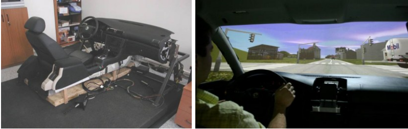
Fig. 24: One of the first prototypes of out light simulator (2003) – left and contemporary look of our light simulator Superb (2007) - right
