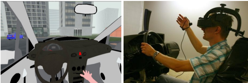
Fig. 27: VR environment seen in HMDs (left) and driver in virtual simulator, HMD - real parts of the cockpit wearing high resolution, extra-large FOV HMD (right)
