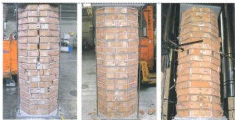
Figure 7 – Columns at the end of the test: (left) plain column, (center) strands in alternate joints, (right) strands in all mortar joints.
