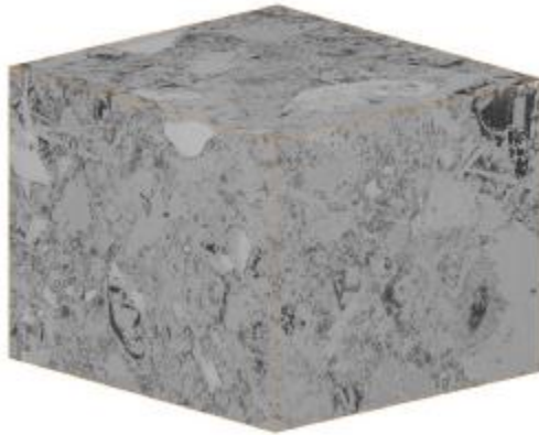
Figure 6 - Three-dimensional dataset of hardened Portland cement paste based on focussed ion beam nanotomography (FIB-nt). The isometric voxel size is 20 nm, leading to the corresponding size of the dataset of 35.2 \times 26.5 \times 32.0 \mu\text{m}^3 .
