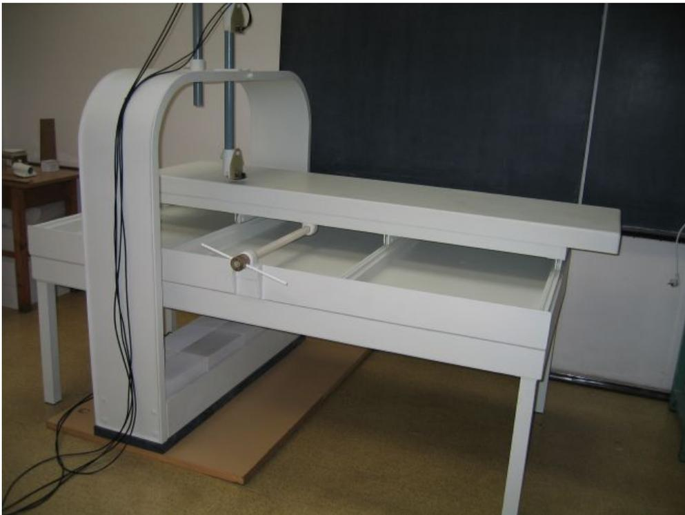
Fig. 4.1 – The nonmagnetic positioning bed for scanning of field maps
