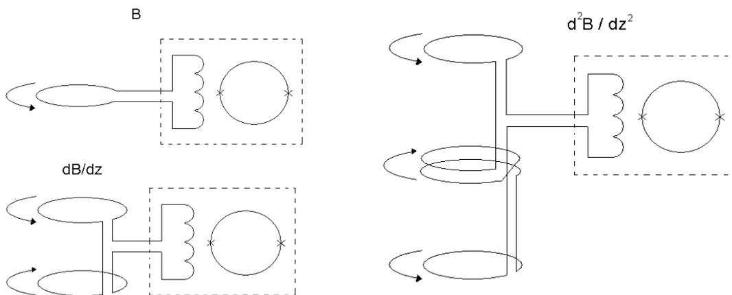
Fig. 2.1 – Superconducting flux transformers used with SQUID. Magnetometer, first-order gradiometer and second-order gradiometer configurations are shown (after [16])
