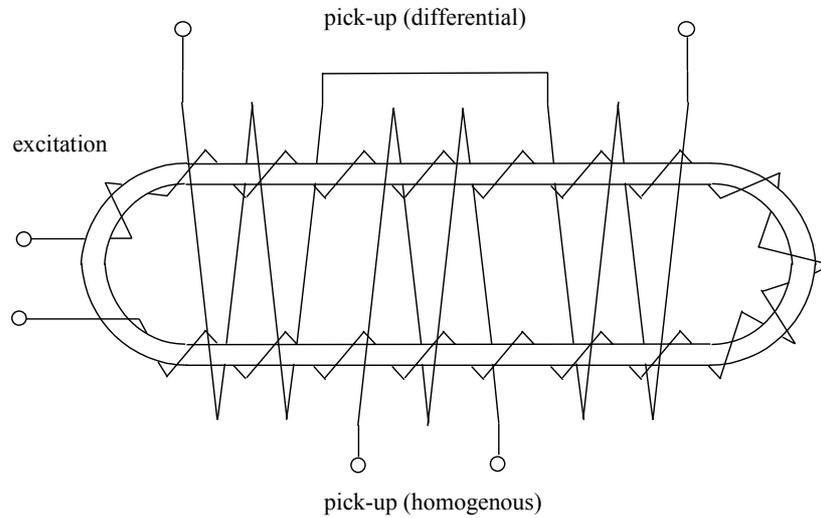
Fig. 3.4 – Race-track core fluxgate with standard (homogenous field) pick-up and (optional) differential pick-up
