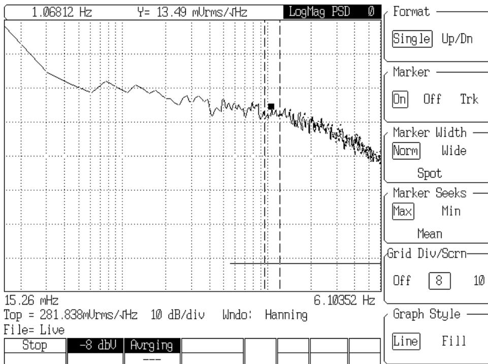
Fig. 3.3 – Noise spectrum (PSD) of single-core differential fluxgate. The gradient sensitivity is about 6.4μT/m/V. The indicated voltage thus corresponds to about 90nT/m/sqrtHz at 1 Hz
