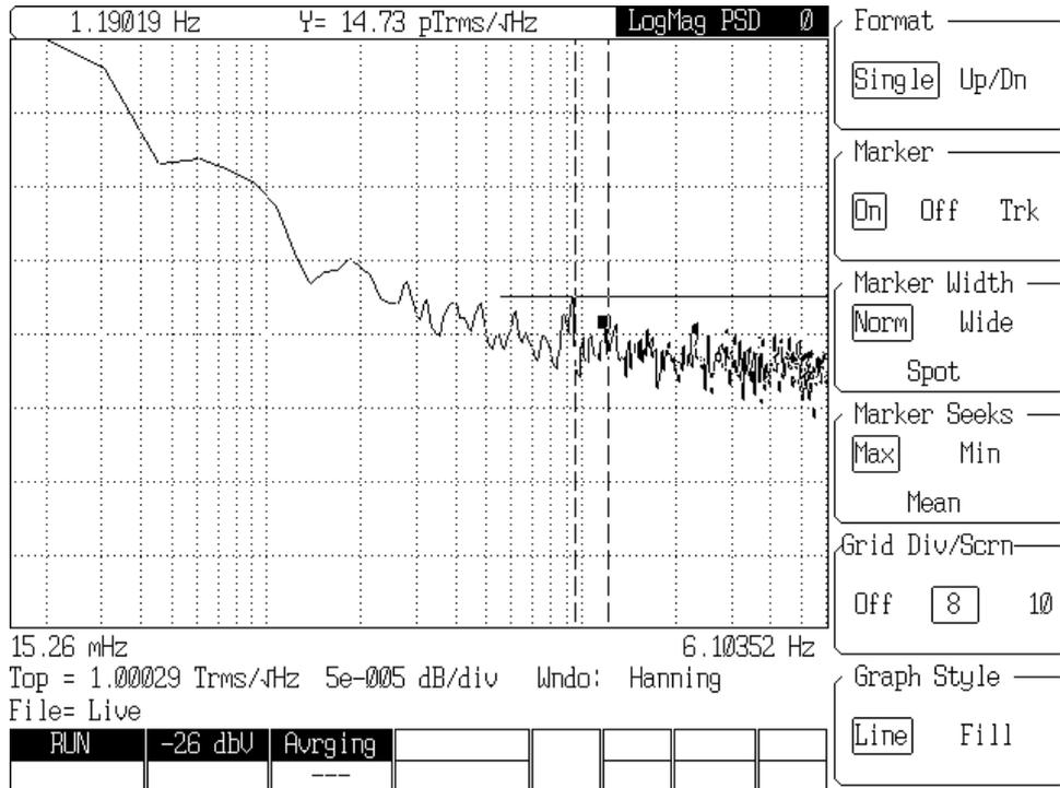
Fig. 3.2 – Noise spectrum (PSD) of ring-core fluxgate sensor in low frequency range. The noise is of 1/f type, about 15pT/sqrtHz at 1Hz
