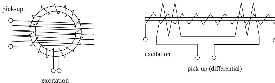
Fig. 3.1 – Ring-core (left) and single wire-core differential fluxgate (right)
