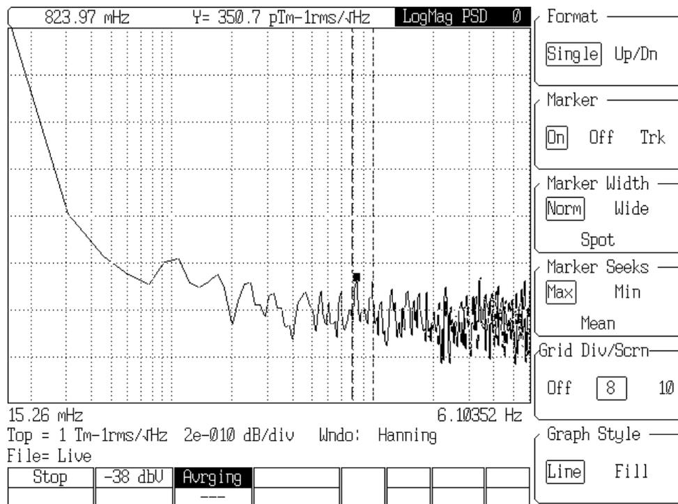
Fig. 3.6 – Noise spectrum (PSD) of gradient signal from two ring-core fluxgates, baseline is 10 cm. The noise is 350 pT/m/sqrtHz at 1Hz.
