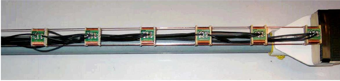
Fig. 4.2 – Fixture with multiple fluxgate sensors forming several first-order gradiometers, each with baseline of 10 cm (from [19])
