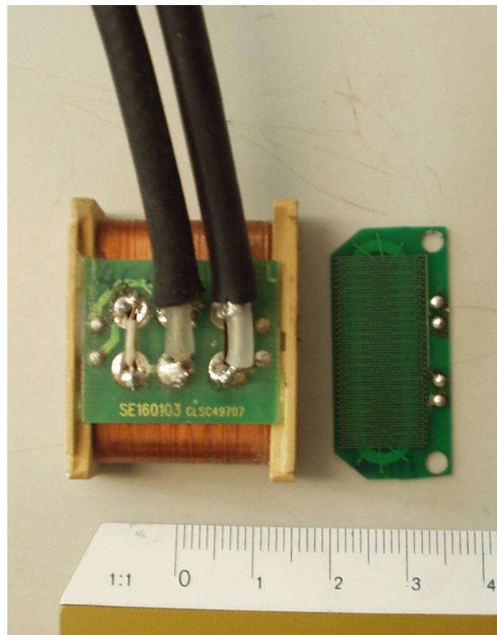
Fig. 3.5 – Ring-core (left) and PCB race-track core (right) fluxgate sensors
