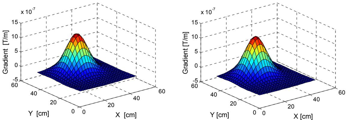
Fig. 4.3 – Comparison of modeled (left) and measured (right) gradient field from a compact source. The closer probe is 18 cm above bed surface, the other is 10 cm further away (from [19])
