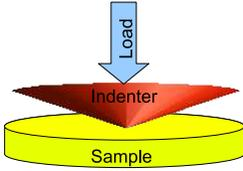
Figure 3: Principle of nanoindentation.
