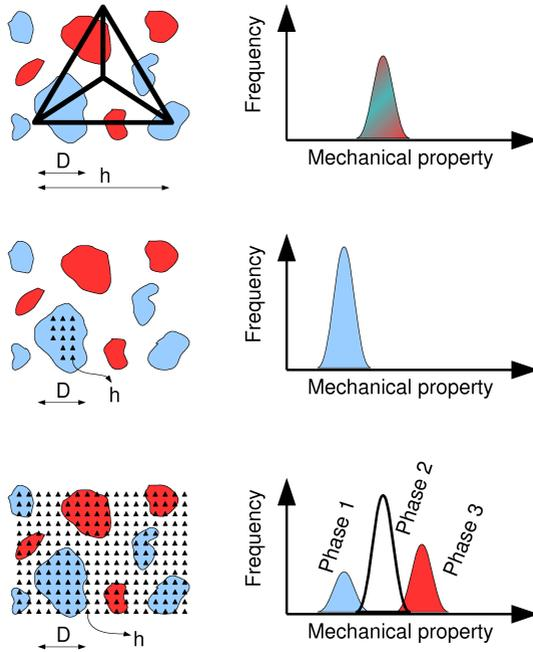
Figure 11: Schematic representation of three testing strategies. Top: Large indent producing average properties. Middle: Small indents pointed into one phase. Bottom: Large grid of small indents produced over large sample area. The overall property histogram is a convolution of results from several phases in this case.
