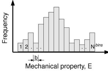
Figure 12: Construction of property histogram with bin size  $b$ .
