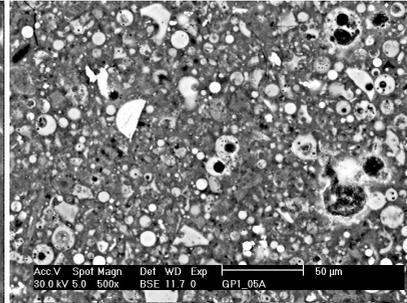
Figure 10: ESEM image of alkali-activated fly ash. Light and light grey areas= unreacted or partly reacted fly-ash grains; dark grey areas= polymer zone; dark areas= pores.
