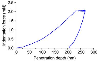
Figure 2: Typical load versus penetration diagram from nanoindentation.
