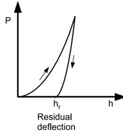
Figure 4: Loading diagram.
