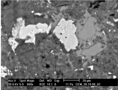
Figure 9: ESEM image of hydrated cement paste. Dark areas= pores; dark grey= C-S-H gels; light grey= Portlandite; light areas= unreacted clinker.
