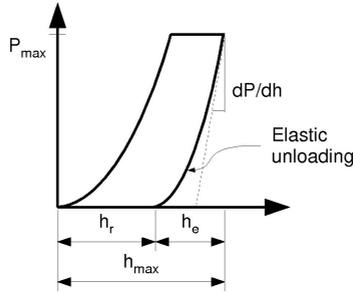
Figure 7: Loading diagram.
