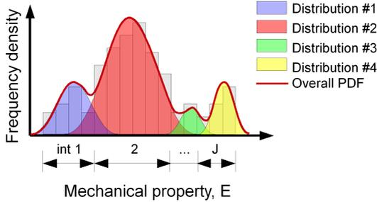
Figure 13: Separation of the experimental dataset to  $j = 1 \dots M$  intervals and construction of  $M$  probability density functions.
