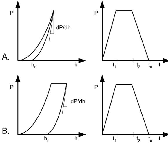
Figure 6: A. Load-depth and load-time plots for elastic-plastic solid, B. Load-depth and load-time plots for visco-elasto-plastic solid.
